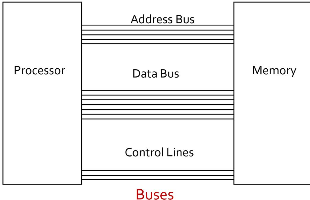
There are 2 **buses** connecting the processor and memory; the **data bus** and the address bus. There is a third connection called the control lines, some people class this as a bus as well.
