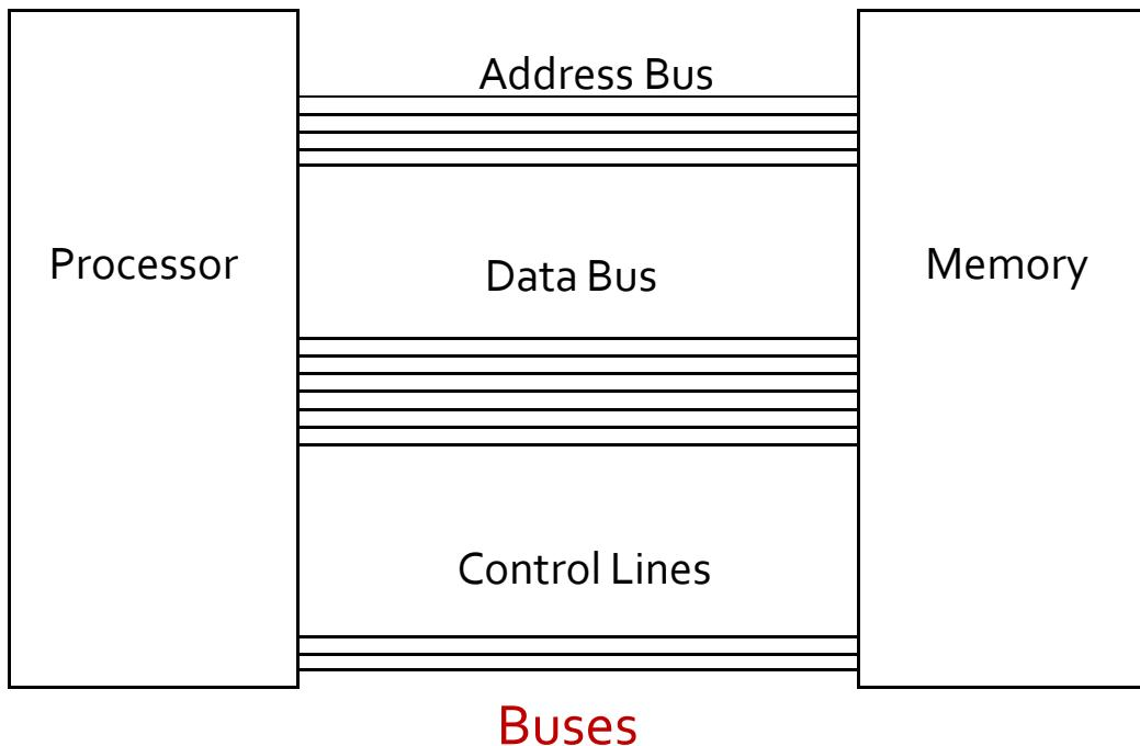
There are 2 **buses** connecting the processor and memory; the **data bus** and the address bus. There is a third connection called the control lines, some people class this as a bus as well.
