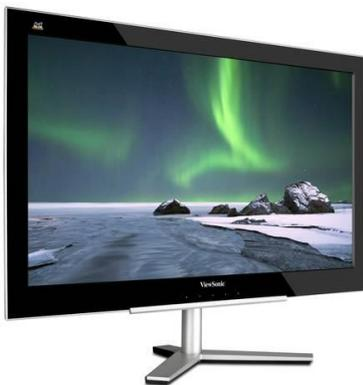
The main output device on every computer you use will be the **monitor** or screen. The monitor is made up of a grid of very small dots called **pixels**. Each pixel can be set to a **different colour** and can change colours quickly. This allows still images and video to be displayed on the monitor.
