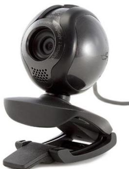
**Webcams** function like very basic digital video cameras. They are generally of very low quality because it is hard to send video across the internet. As Internet speeds have increased the resolution of webcams has also increased.
