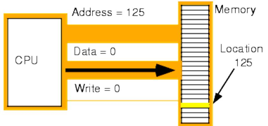
Note - The address bus is one directional as it only ever sends address information from the processor to the memory. The data bus is bi-directional as data can travel to and from the processor.
