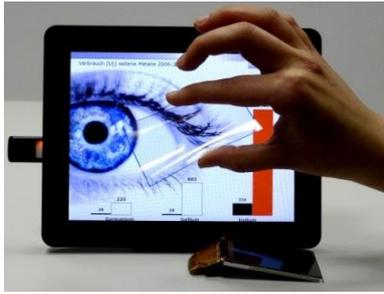
As smartphones and tablets have become more popular the use of **touch screens** as input devices has increased. A good **touchscreen** can combine the benefits of keyboards and track pads by using **virtual keyboards** that are displayed on the screen.
