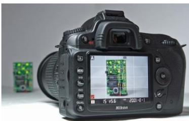
**Digital cameras** use an array of sensors to capture pictures which can be inputted into a computer. The quality of a picture is usually measured by the resolution of the camera; this is normally given in megapixels.
