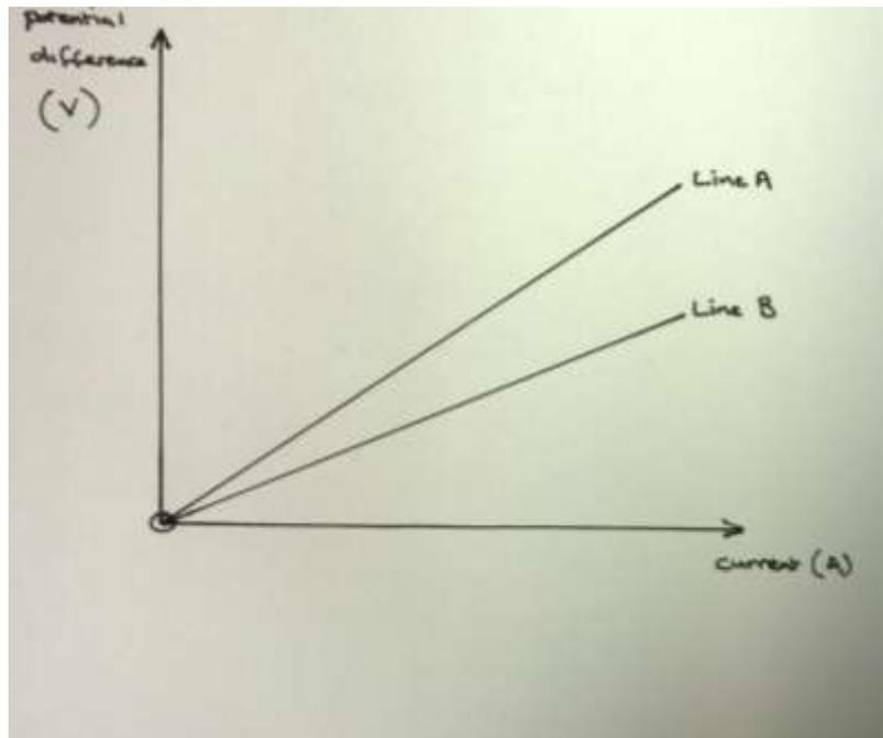
Which line on the graph represents the results for the 10 ohm resistor?
